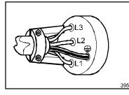
A 4 pole plug, suitable with the current socket, must be installed at the end of the device's power supply cable.
